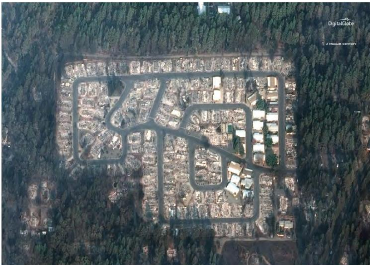
Camp fire, showing devastation of homes in the Kilcrease Circle community of Paradise, a contrast to the green mature forest, with little or no scorching, which surrounds this neighborhood. The homes here were not burned by high-intensity crown fire, but rather were burned when embers driven on the winds landed on flammable homes followed by home-to-home ignitions. Courtesy Satellite image ©2018 DigitalGlobe, a Maxar company/Handout via REUTERS, Nov. 17, 2018.
